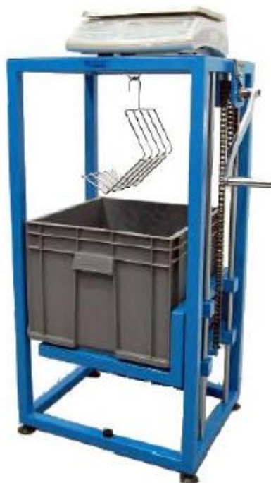
Figure 2. Determination of density by hydrostatic weighing.
