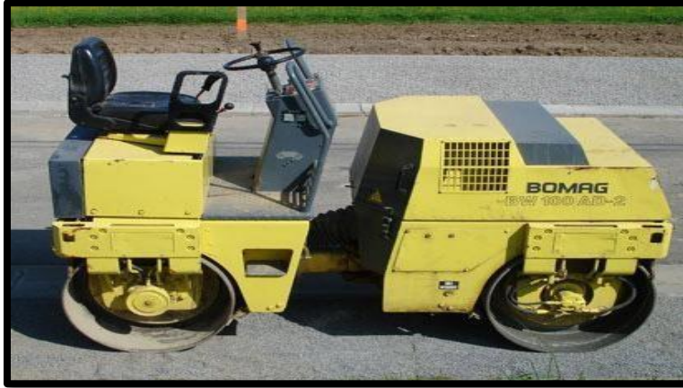
Figure 3. 8. Roller compactor (2.5t).
