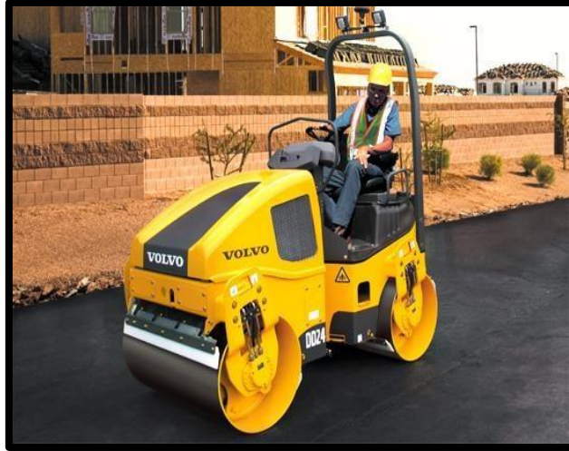
Figure 3. 10. Vibratory roller (1.5 to 3.8 t).
