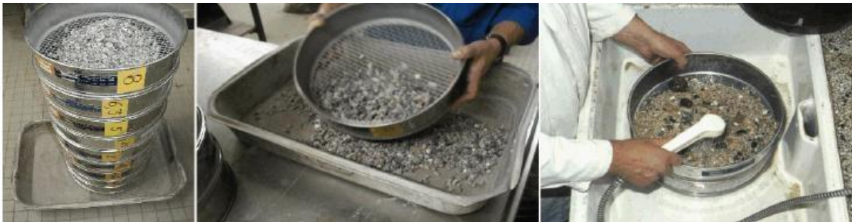
Figure 2. 4. Different phases of granulometric analysis by sieving.
