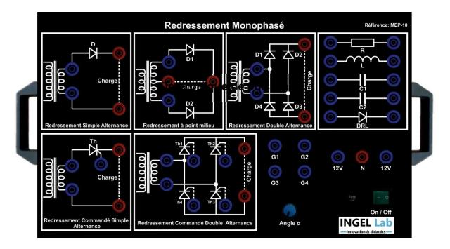
The model is powered by a 15V midpoint transformer and allows the following educational operations:
