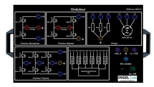
The model is equipped with a variable DC power supply -12V...0...+12V and allows the following educational operations:
